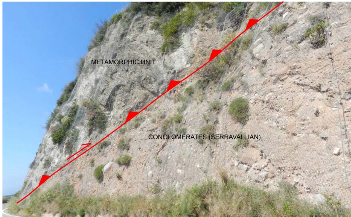
Fig. 33 – Tectonic contact between the basal conglomerates of the first stratigraphic sequence (Serravallian) and the metamorphic substrate (Paleozoic).
